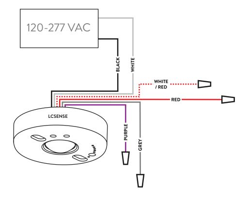
**Switched Neutral:** The "Switched Neutral" white with red stripe wire is the neutral line for the load being switched. This enables power measurement.
