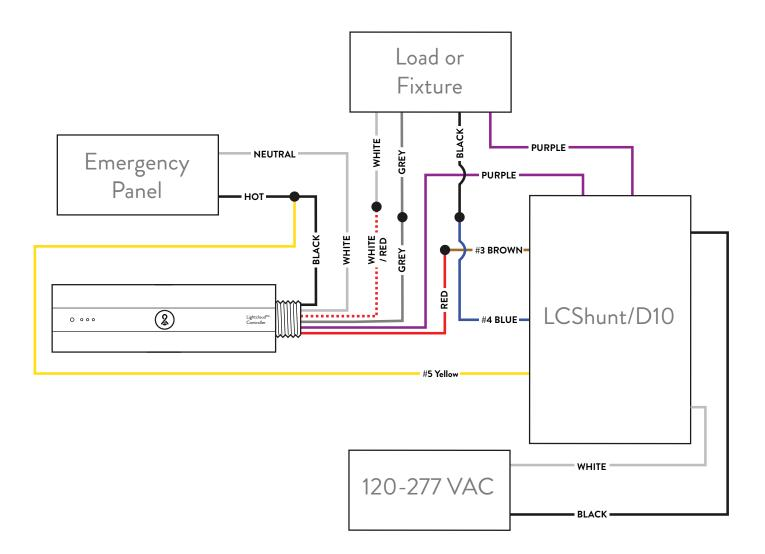
**Note:** The LCSHUNT includes a 20A rated high voltage Form C (N/O+N/C) relay and a low voltage Form A (N/O) relay and is UL924 Listed for emergency
