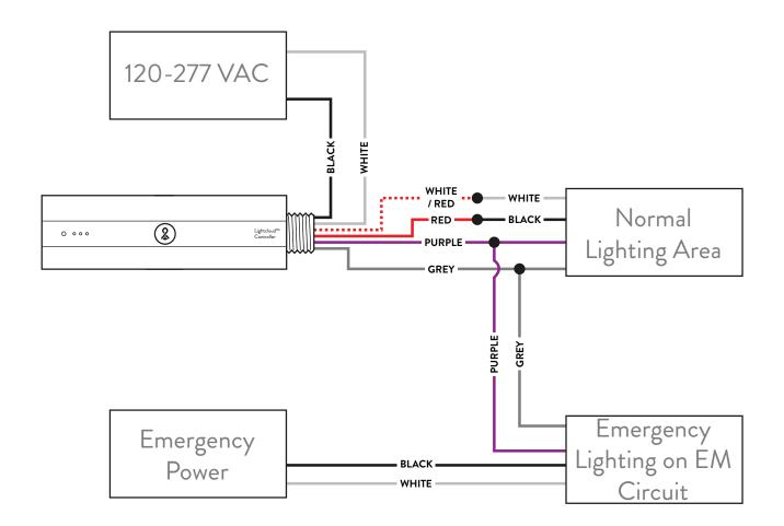
**Notes:** In spaces where there is only one luminaire, and it is connected to emergency power, the Controller will need to be connected to a Normal Power Circuit for proper operation. Emergency fixtures with on-board battery backup don't require special wiring.
