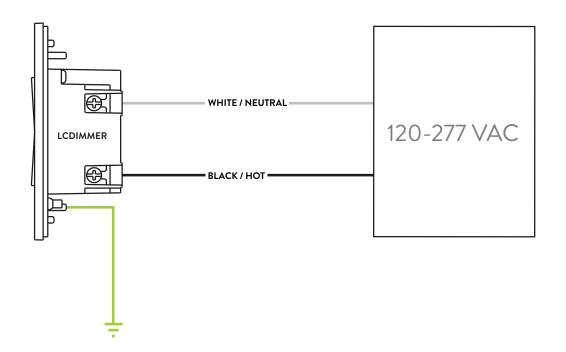
Input: 120-277VAC, 50/60Hz, 2W 18AWG grounding; terminals supporting up to 12AWG wire
