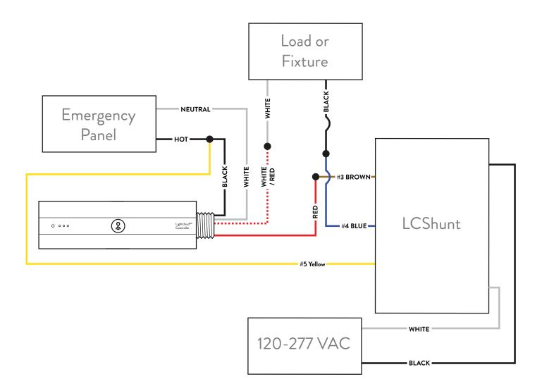
**Note:** The LCSHUNT includes a 20A rated high voltage Form C (N/O+N/C) relay and is UL924 Listed for emergency lighting control applications. The LCSHUNT can bypass a line voltage switch or dimmer, ensuring that an emergency fixture illuminates at full brightness during a utility power interruption.
