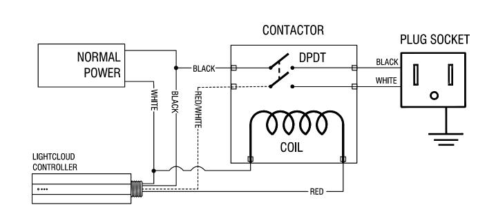
PLUG LOAD CONTROL: LIGHTCLOUD CONTROLLERS CAN BE USED TO CONTROL POWER TO RECEPTACLES THROUGH A CONTACTOR. CONTACTOR BY OTHERS. **INSTALLATION:** ANY WIRES NOT IN USE MUST BE CAPPED OFF OR OTHERWISE INSULATED. THIS PRODUCT SHOULD ONLY BE INSTALLED BY A QUALIFIED ELECTRICIAN AND IN COMPLIANCE WITH LOCAL AND NATIONAL ELECTRICAL CODES.
