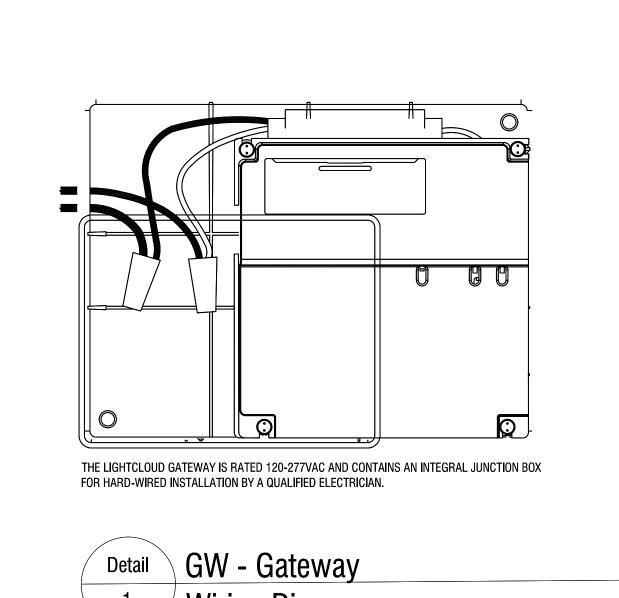
THE "SWITCHED NEUTRAL" WHITE WITH RED STRIPE WIRE IS THE NEUTRAL LINE FOR THE LOAD BEING SWITCHED. THIS ENABLES POWER MEASUREMENT.
