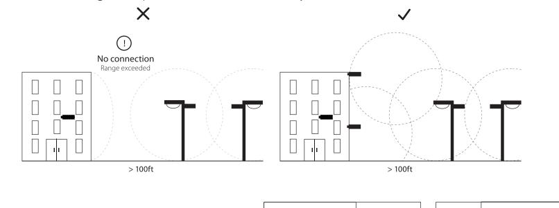
**Device Around Corners** If you need to direct a wireless mesh signal around the corner of a building, you can install two Controllers in a 90° fashion from each other as pictured.
