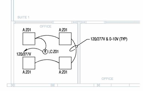
One LC Controller can control up to 15 Amps of load. In this scenario, we are using one LC Controller to control all the fixtures in the office. This will minimize device quantities, but the 0-10V control wiring will need to be daisy chained to each fixture as well as power wiring if dimming is desired.
