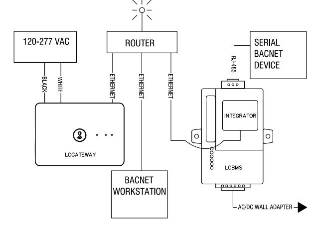
INTEGRATOR: INTEGRATOR INPUT SHALL BE 9-30 VDC OR 12-24 VAC. **GATEWAY:** THE GATEWAY SHALL BE HARDWIRED TO A 120V POWER SUPPLY. INSTALLATION: ANY WIRES NOT IN USE MUST BE CAPPED OFF OR OTHERWISE INSULATED. THIS PRODUCT SHOULD ONLY BE INSTALLED BY A QUALIFIED ELECTRICIAN AND IN COMPLIANCE WITH LOCAL AND NATIONAL ELECTRICAL CODES.
