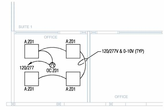
One OC can act just line and LC Controller, and can control up to 15 Amps of load. In this scenario, we are using one OC to control all the fixtures in the office. The OC can be programmed as both Occupancy and Vacancy Sensing. This will minimize device quantities, but the 0-10V control wiring will need to be daisy chained to each fixture as well as power wiring if dimming is desired.
