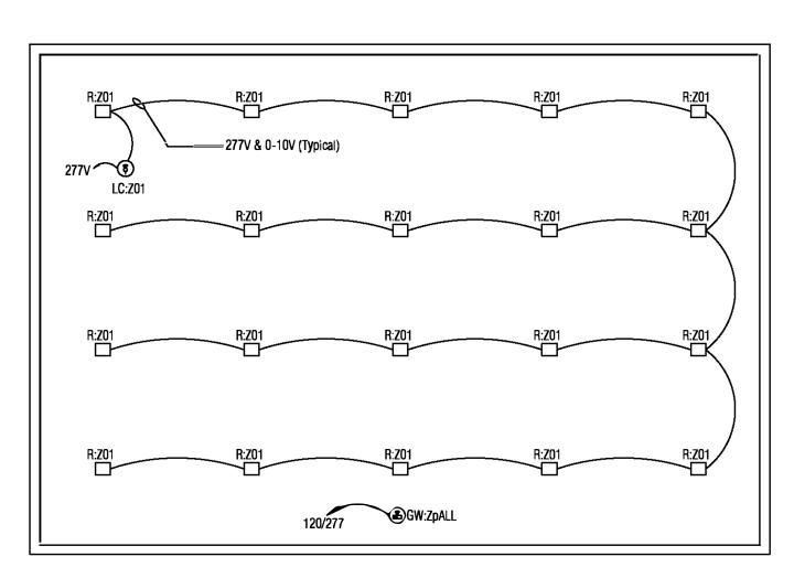
This scenario uses the least amount of devices possible. One LC Controller can accommodate all up to a 15A load so if we assume that these fixtures are RAIL150's and they are fed with 277V, we can control all luminaires as one zone. The LC Controller can be mounted anywhere or onboard the first fixture. This will minimize device quantities, but the 0-10V control wiring will need to be daisy chained to each fixture as well as power wiring if dimming is desired.
