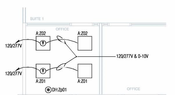
Two Zones could be provided by adding an LC Controller on-board two of the fixtures then daisy chaining the 120/277V and 0-10V Control wiring to the second fixture. This would be a good choice when using the Daylight Harvester. In this case, the two fixtures adjacent to the windows could be one Zone, and the other two can be a second zone.
