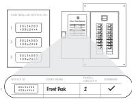
For setup and maintenance, we provide two Lightcloud Device Tables with the Gateway: one that you can attach to your panel and one to hand off to a building manager. Attach the Device Identification stickers included witheach device to a row, then write in additional information, such as Zone name, Panel/Circuit Number, and whether or not a zone uses dimming.
