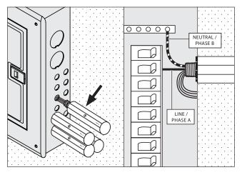
Space and code allowing, you may install Lightcloud devices directly in your breaker box or lighting panel. Alternatively, break out lighting circuits and install Lightcloud devices in a separate trough.
