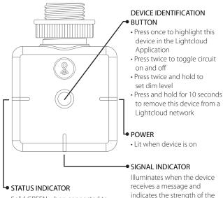
Solid GREEN when connected to your Lightcloud network. Blinking RED when not connected. The device will automatically continue trying to connect to a network in Setup Mode.
