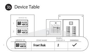
For setup and maintenance, we provide two Lightcloud Device Tables with the Gateway: one that you can attach to your panel and one to hand off to a building manager. Attach the Device Identification stickers included witheach device to a row, then write in additional information, such as Zone name, Panel/Circuit Number, and whether or not a zone uses dimming.
