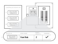
For setup and maintenance, we provide two Lightcloud Device Tables with the Gateway: one that you can attach to your panel and one to hand o" to a building manager. Attach the Device Identification stickers included witheach device to a row, then write in additional information, such as Zone name, Panel/Circuit Number, and whether or not a zone uses dimming.
