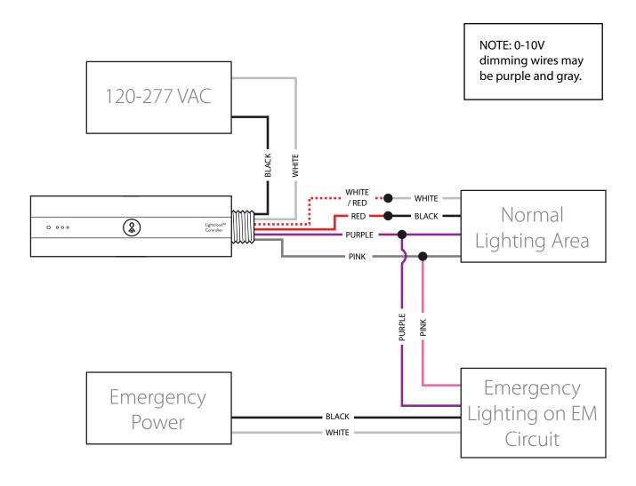
**Notes:** In spaces where there is only one luminaire, and it is connected to emergency power, the Controller will need to be connected to a Normal Power Circuit for proper operation. Emergency fixtures with on-board battery backup don't require special wiring.
