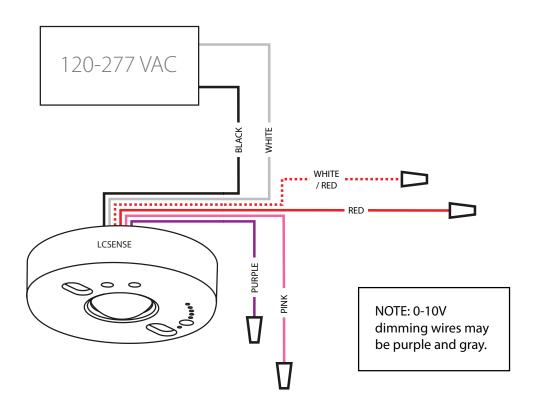
**Switched Neutral:** The "Switched Neutral" white with red stripe wire is the neutral line for the load being switched. This enables power measurement.
